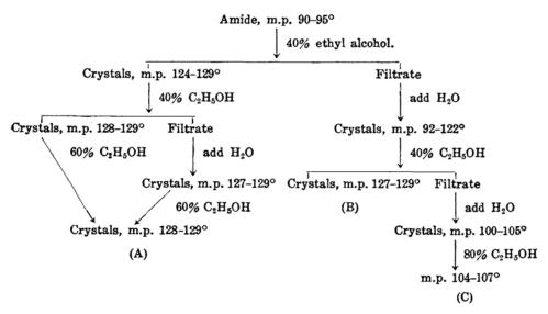
Crystals (A) and (B) were found to be dihydroshonanic amide by examination of the melting points of various mixtures, while crystals (C) was proved to be crude isoshonanic amide.
